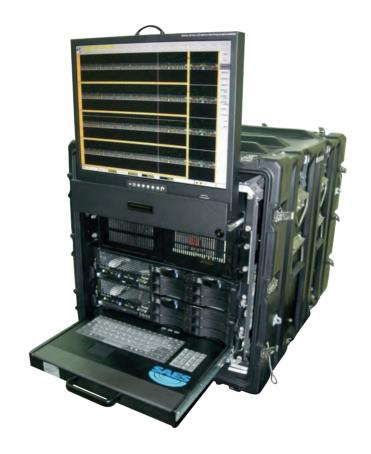
SAES has developed a FTAS to support Maritime Patrol ASW operations. FTAS provides post-mission acoustic signal analysis and intelligence gathering by means of replaying and processing simultaneously the acoustic signals recorded during operation.
