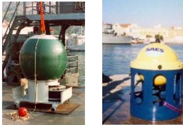
Figure 2. MO-90 moored mine (left) and UMIMS (right).
