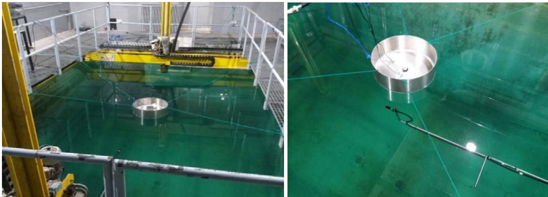
Figure 4. Fixing of the structure in the centre of the water tank (left) and detailed view of the hydrophone positioning (right).
