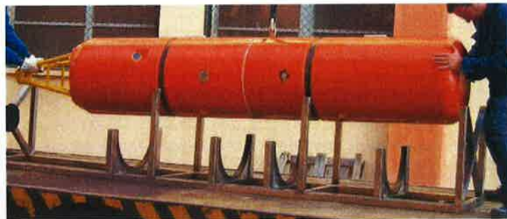
Figure 3. Cylindrical bottom type of advanced MINEA mine.
