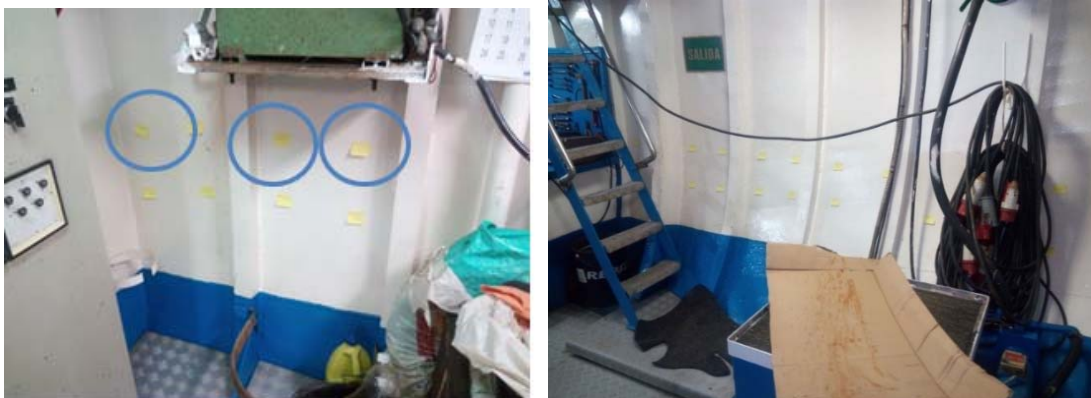
Figure. 4: Measurement points on the 'Manuela Lloret' with hull of steel. Thirty-six (36) points under water line.
