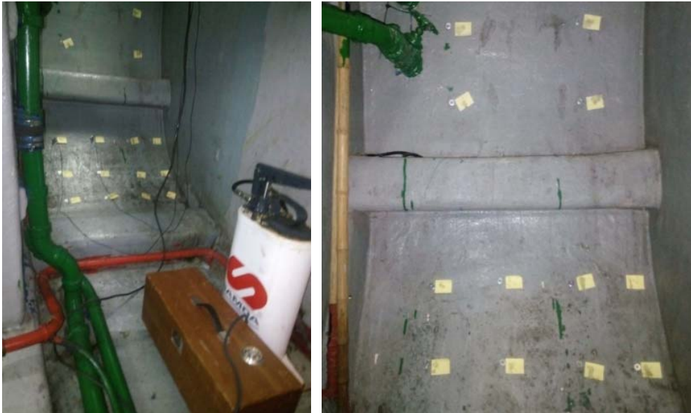
Figure. 3: Measurement points on the 'Verdú Verdú' with hull of GRP. Twelve (12) points under water line and four (4) points above water line.
